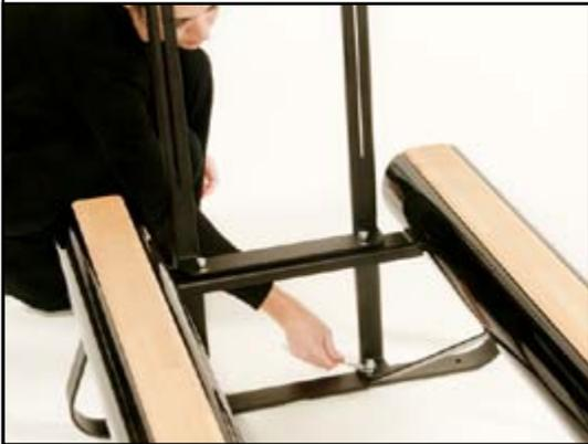
9) Tighten the bottom nuts as well, then fully tighten all the nuts.
