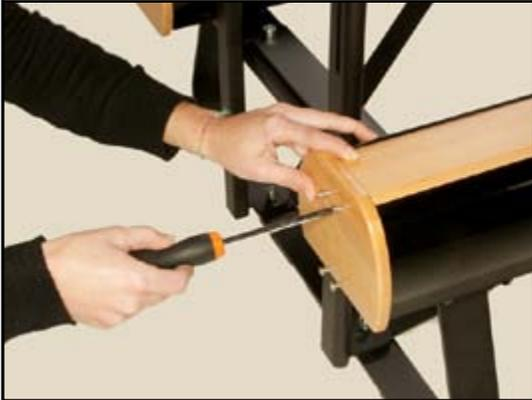
33) Screw the wooden covers, making sure that the shaped section matches the shape of the guards.
