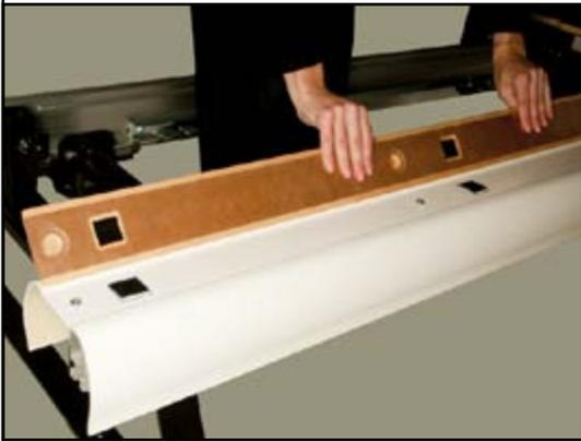
34) Reposition the wooden slats so that they match the position of the frame (bolts, Velcro etc).
