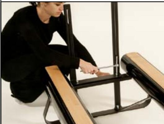
8) Refit the bolts in their housing and fix the risers unit at the same time. Partly tighten the top nuts.
