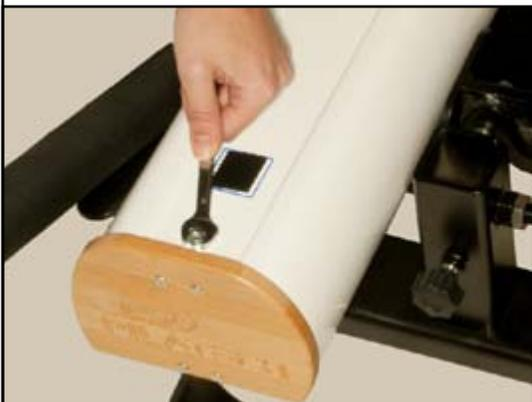
25) Unscrew the bolts on the top sections of the guards.
