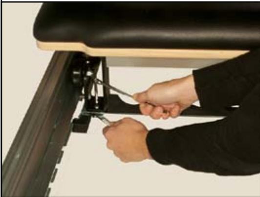
27-28) Unscrew and remove the front spring carrier rod by unscrewing the right and left bolts.
