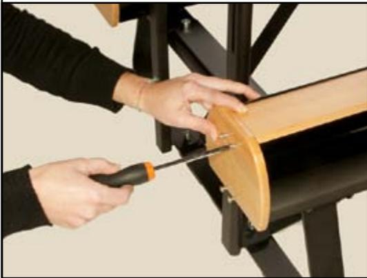
36) Unscrew and remove the two rear wooden covers and remove the top wooden slats.
