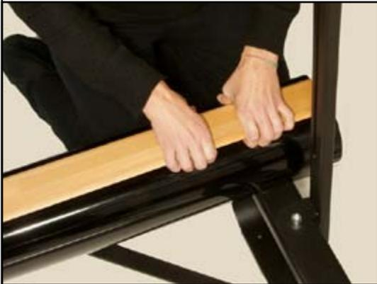
23-24) Apply pressure with your fingers and remove the top wooden slats with great care to prevent any damages.
