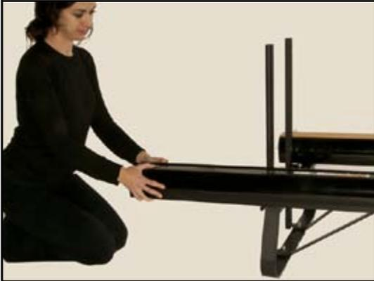
26) Remove the guards from the beams by carefully pulling them width-wise and place them on a safe and level surface, away from rough and sharp parts that could damage them.
