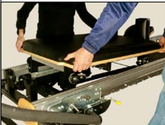
29) Remove the carriage and place it in a safe and level surface, taking care not to damage it.
