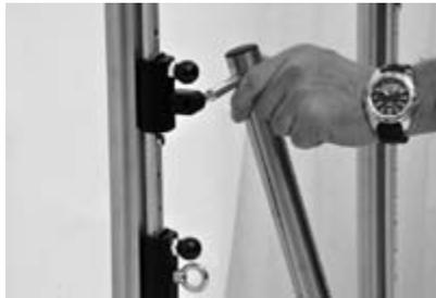
The pin, spacer and locking nut must be fitted in the sequence shown in the picture.
